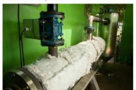
Unlike conventional German biofuel vehicles, the Pyroformer does not need a constant waste stream, different wastes can be entered at the same time and it has been tested with 20 - 30 different waste streams
